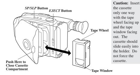
Before inserting a cassette, turn the tape wheel on the side of the cassette in the direction shown to remove any slack in the tape.
